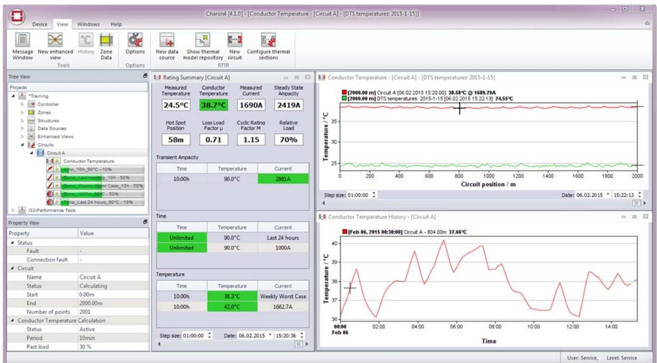
Charon4 visualization showing tree view, conductor temperature job properties, rating summary, conductor temperature profile and conductor temperature history windows
