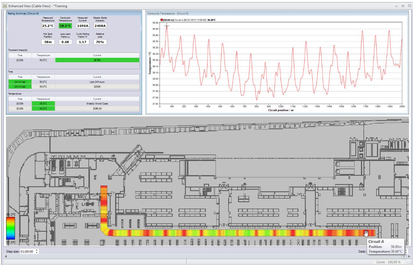
Enhanced View of a power cable installation showing the rating summary, the conductor temperature profile and a drawing of the installation with a false colour representation of conductor temperature along the cable
