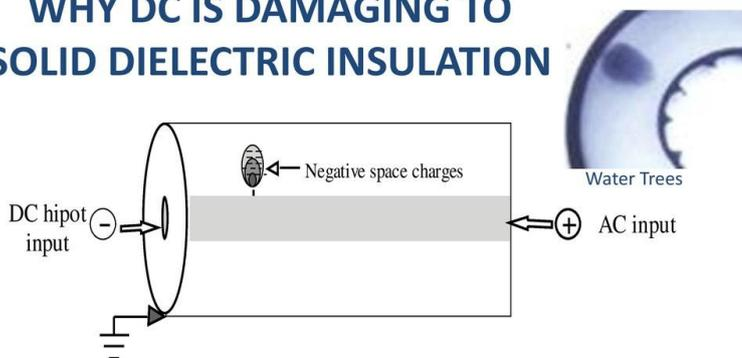
The 4 – 5  $U_0$  negative output of a DC hipot test polarizes water tree areas.
