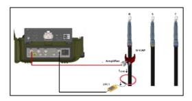
**HFCT sensors** should be used if the termination earth straps are available. The HFCT sensors are more sensitive and permits assessments of long run cables.
