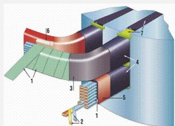
Almost all medium and high voltage motor and generator stator windings rated 6 kV and above have coatings on the surface of the coils or bars to suppress the occurrence of partial discharges (PD) on coils or bars operating at high voltage.
