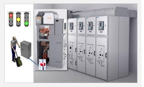
Partial Discharge sensors must be fitted on the bottom of the cable terminations. The sensors will be connected to the In-Time monitor that will detect and trend electrical discharge pulses D(PD).
