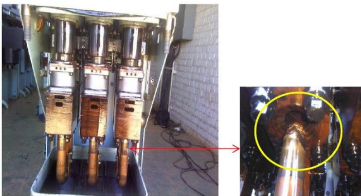
Contact welding can occur in situations where the fault currents are very high and where DC offset transients occur as these will generate substantial electro-dynamic forces on the contacts. This occurs because of the constriction of current streamlines which occurs at contacts and particularly at switching contacts. The constriction results in an electrodynamic
