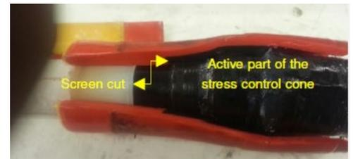
Incorrect installation of the stress control will lead to tracking type discharges and premature failure.
