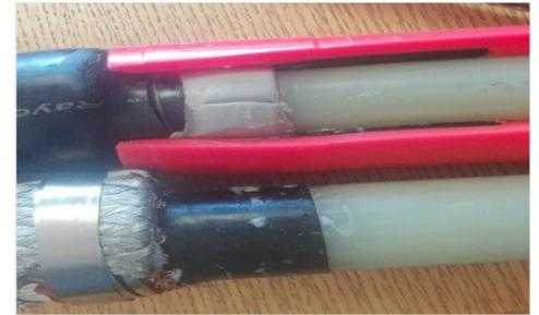
The active part of the stress cone was not in the correct place and did not make contact with the screen cut.
