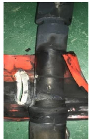
Creepage distance is incorrect that create tracking inside the termination and lead to failure
