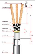
**Step 2:** Martec QC record the dimensions accordingly and ensure that the stress control system is in the correct position.
