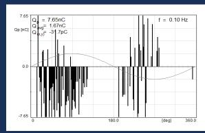
PD levels of up to 3825pC were detected coming from the cable terminations.
